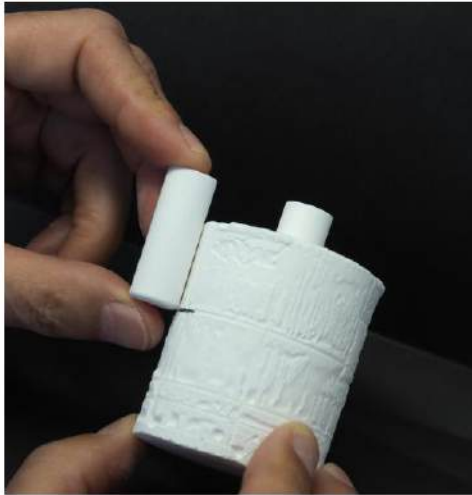
mark the position of plunger on the outside of the investment ring
