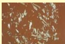
White gold particles have a positive influence on the flow behavior of the solder.
