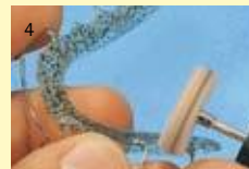
The three layers of felt adapt to any type of structure so that even very fine polishing is simplified.
