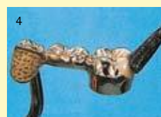
Shake the Oxyd-Stop-PM well and brush it onto the areas to be protected. Allow briefly to dry. The surface is now optimally protected against oxidation.
