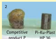
At 275°C the competitor's product foams and expands considerably.
