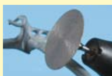
Separating and grinding back the sprues.
