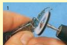
Fabric discs that have been soaked with polishing paste polish more smoothly. This saves time because it is not necessary to apply polishing paste.
