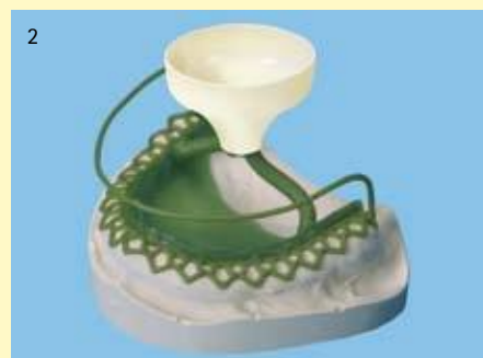
2 During casting the compressed air is displaced into the air channels and produces castings free from shrinkage cavities, which can be easily fitted.
