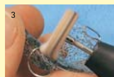
The three-layer felt buff polishes clasp transitions gently and quickly.
